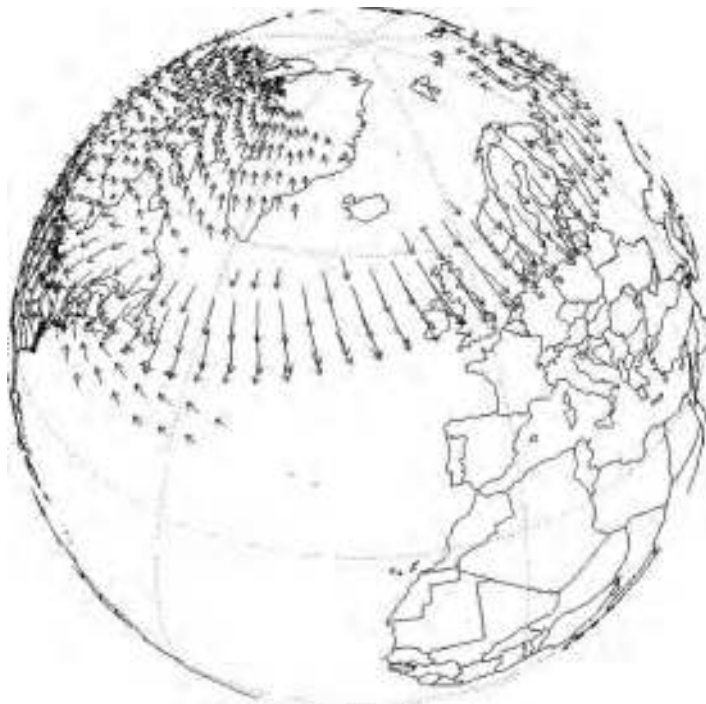
FIGURE 16.16 Extensive westward electrojet-driven geomagnetic field disturbances at time 22:00 UT on March 13, 1989.
