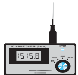
FIGURE 15.6 Typical magnetometer. (Photo courtesy AlphaLab, Inc.)
