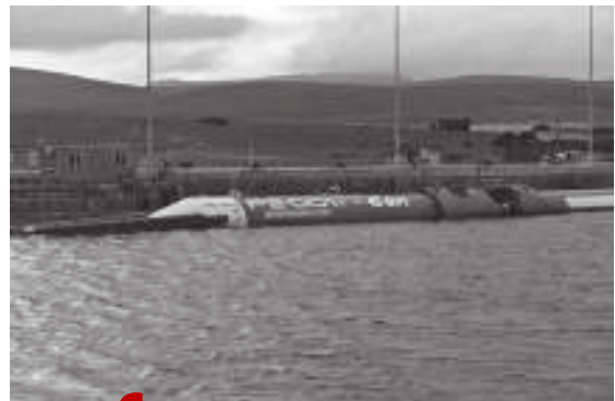
FIGURE P9.52 Pelamis P-750 wave energy converter. Used with permission from © Doug Houghton (Jamy)
