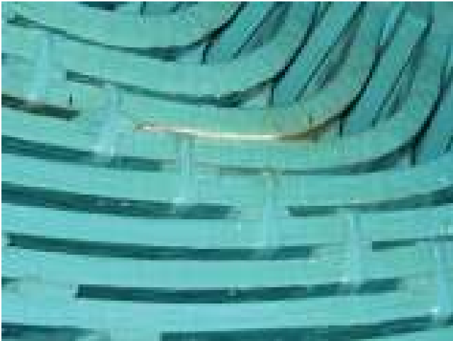
Figure 8.20 PD between adjacent coils in different phases results in white powder on the stator bar surfaces.
