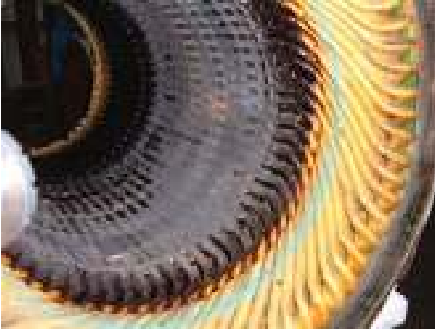
Figure 13.1 Blockage of stator core ventilation ducts with dirt and oil.
