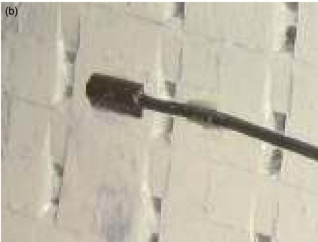
Figure 16.13 (a) A photo of a conventional wedge-mounted foldable flux probe that projects into the air gap. (b) A photo of an installed flat flux probe glued to a stator tooth. (Source: Iris Power-Qualitrol.)
