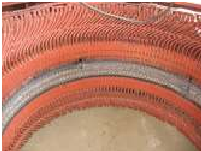
Figure 13.6 Large slow speed motor stator rub from rotor pull over the rub is in the middle of the stator core, at the lighter colored area.
