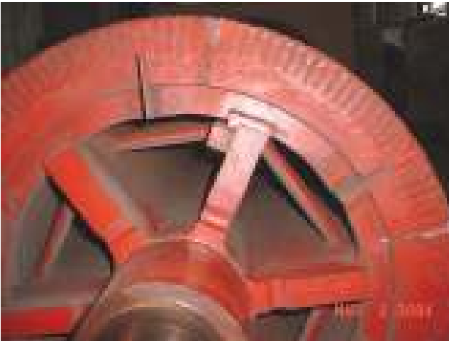
Figure 12.6 Cracks in shorting ring of high inertia drive motor due to low cycle fatigue.
