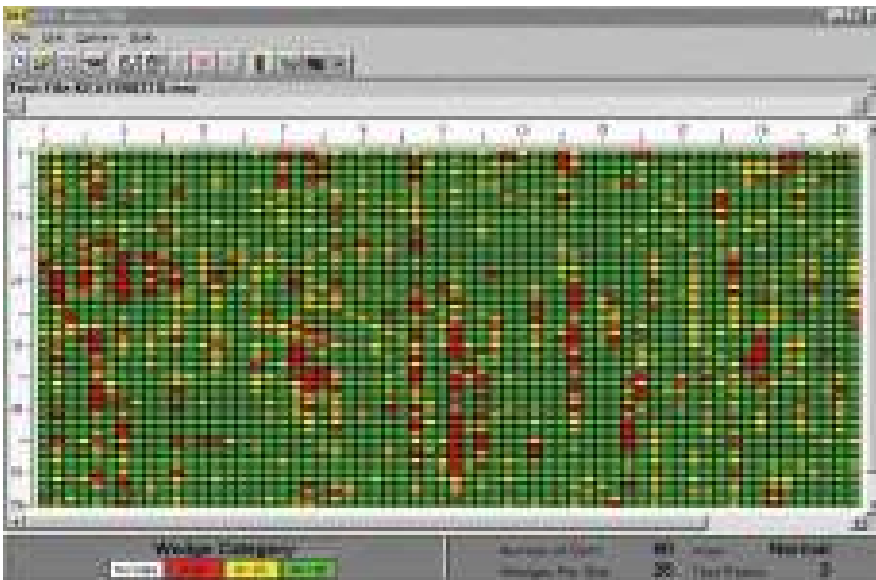
Figure 15.9 Map of wedge tightness versus slot number (vertical scale) and axial wedge number (horizontal scale). Green is tight, red is loose, and yellow is indeterminate. (Source: Iris Power-Qualitrol). See color plate section.
