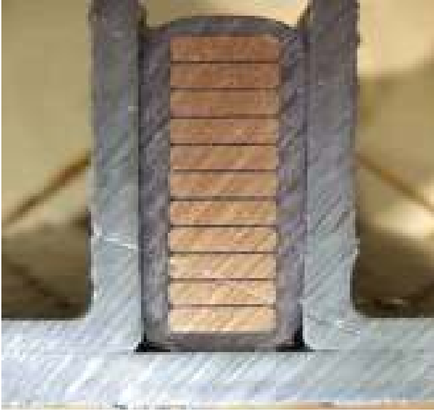
Figure 18.5 Section of sample global VPI'd coil in simulated slot.
