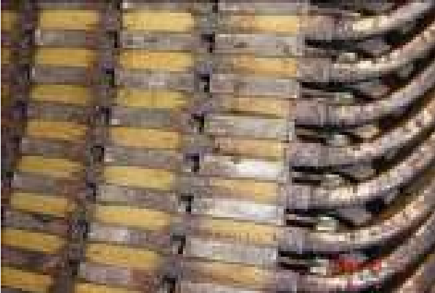
Figure 8.18 Photo of a stator winding degraded by acids in chimney flue gas. (See color plate section).
