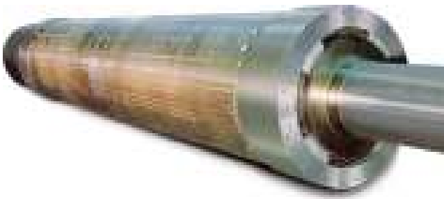
Figure 1.2 Photograph of a round rotor. The retaining rings are at each end of the rotor body.
