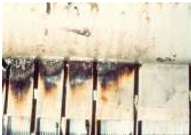
Figure 13.12 Back of core burning at key bar.
