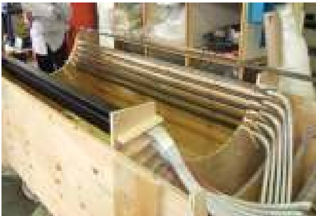
Figure 18.3 Stator core mockup to check bar fit and endwinding spacing.
