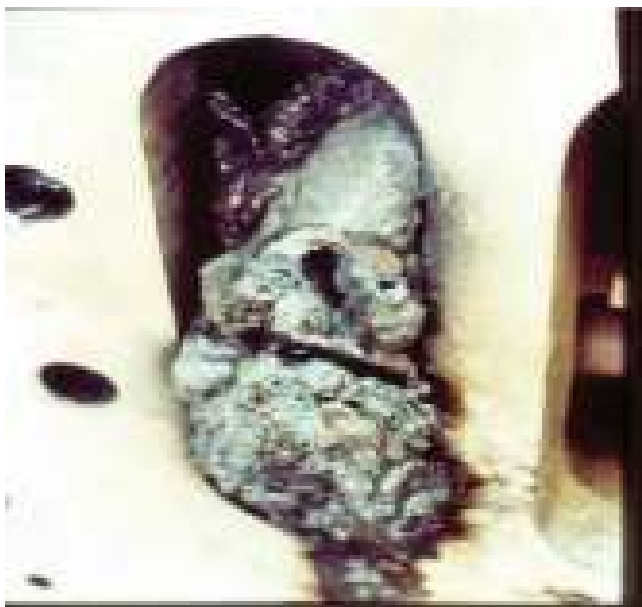
Figure 13.8 Massive core melting with molten steel coming out of the axial vent ducts in a large turbo generator.
