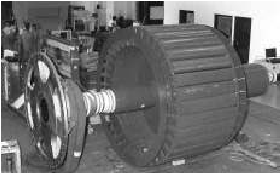
Figure 1.3. Photograph of a salient pole rotor for a large, low-speed motor. (Courtesy TECO-Westinghouse.)
