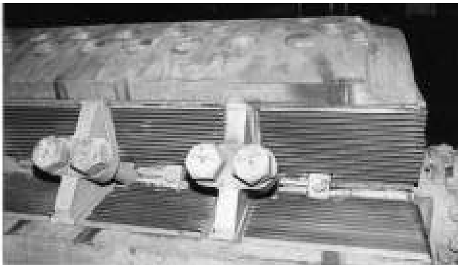
Figure 1.19. Photo of a pole on a salient pole rotor. The V block is between two adjacent poles.
