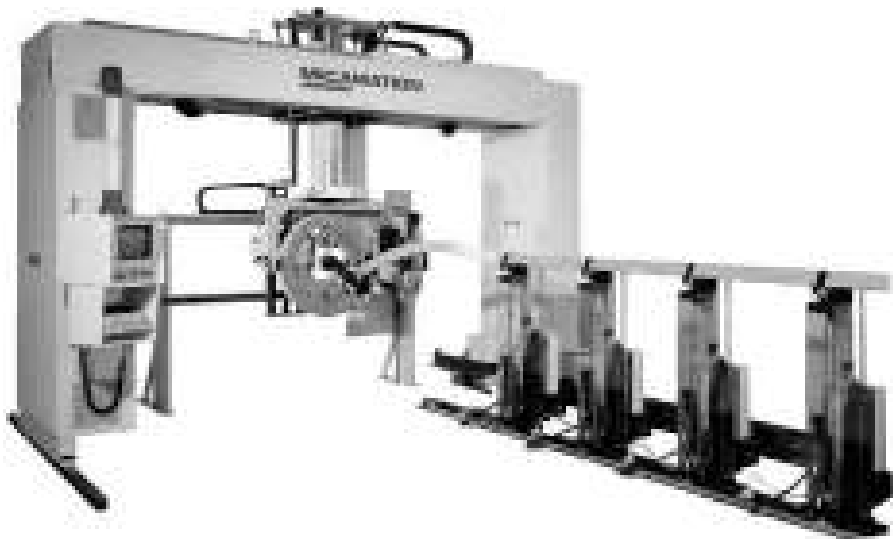
Figure 4.1. A modern stator bar taping machine that applies the tape both in the slot and end-winding portions of the bar.
