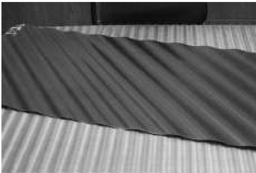
Figure 1.16. Photograph of semiconductive ripple spring material lying on top of nonconductive ripple spring material.
