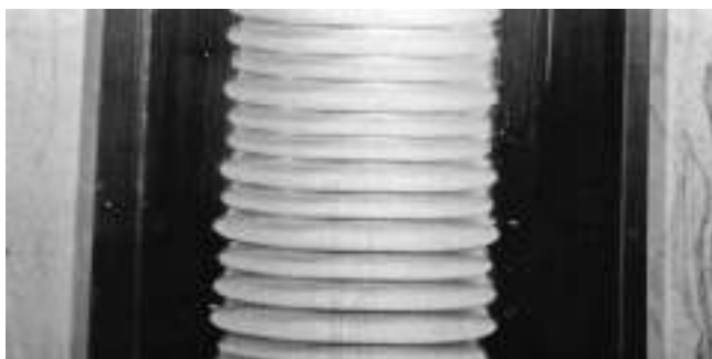
Figure 13.18 The photomicrograph of a damaged bearing race showing fluting brought about by discharge bearing currents (magnified 7 times). The term fluting refers to a regular pattern similar to the pattern eroded into lakeshore sand by wave motion. In this case, steel erosion is brought about by continual electrical discharge. In the photograph, the dark areas show undamaged steel. The lighter flutes represent damage. Source: Reproduced with permission from ABB.
