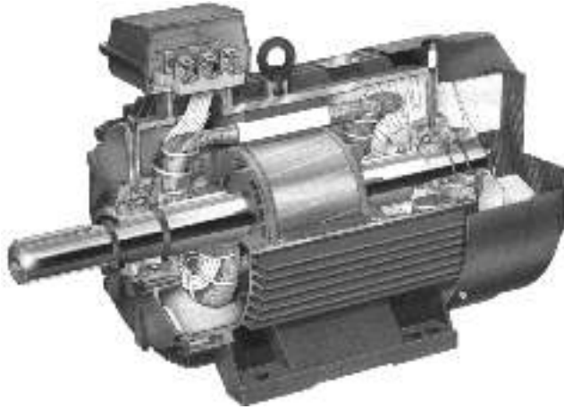
Figure 11.1 Totally enclosed ABB M2BA 280 fan-cooled motor (shaft height 280 mm), 75 kW, 3000 rpm. The rotor squirrel-cage bars are barely visible. The squirrel-cage end rings are equipped with cooling fan blades. The stator features a standard distributed three-phase winding with all six ends brought to the connection box enabling delta or star connection. Source: Reproduced with permission from ABB.
