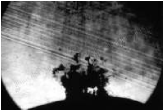
FIGURE 19.11 Water tree and electrical tree. Photo by W. A. Thue.
