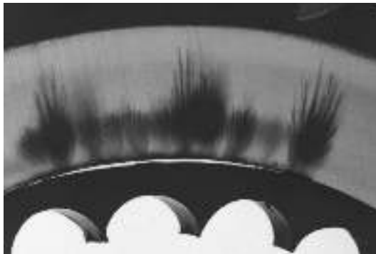
FIGURE 19.4 Vented water trees growing from a loose extruded strand shield in a 175-mil wall of XLPE cable.
