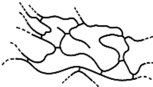
FIGURE 5.10 Cross-linked polymer showing coiled chains.
