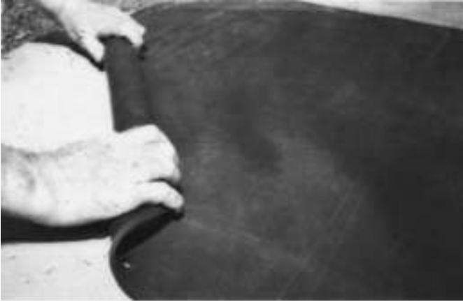
FIGURE 2.21 Inspection of rubber blanket by rolling. ( Courtesy ASTM. )
