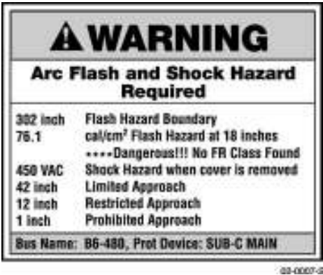
FIGURE 5.2 Preferred required warning label for posting on electrical equipment to warn of hazards.
