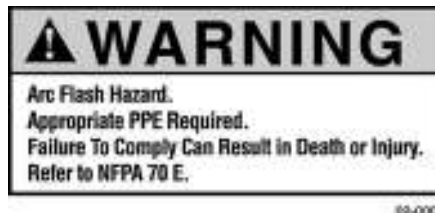
FIGURE 5.1 Minimum required warning label for posting on electrical equipment to warn of hazards.
