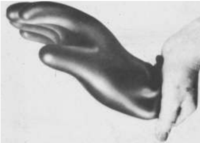
FIGURE 2.25 Visually inspecting inflated rubber gloves. ( Courtesy ASTM. )
