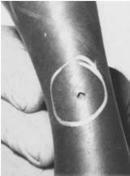
FIGURE 2.36 Nick. (Courtesy ASTM.)
