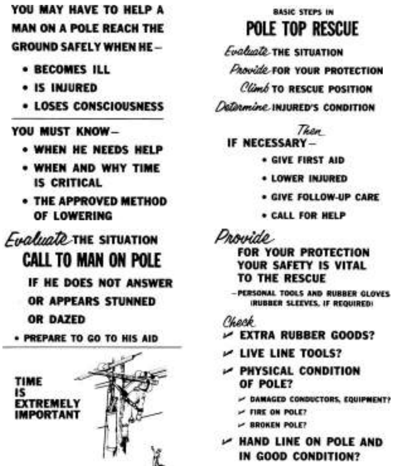
FIGURE 7.8 Illustrated method for elevated, pole-top rescue.
