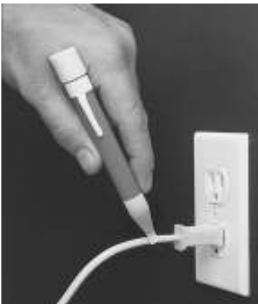
FIGURE 2.58 "AC Sensor" proximity voltage sensor for use on circuits up to 600 V alternating current. (Courtesy Santronics, Inc., Sanford, NC.)
