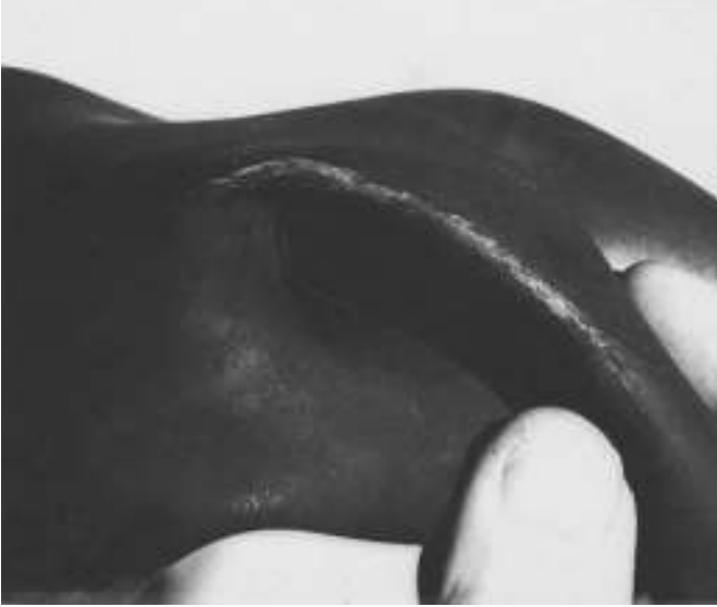
FIGURE 2.28 Age cracks. (Courtesy ASTM.)
