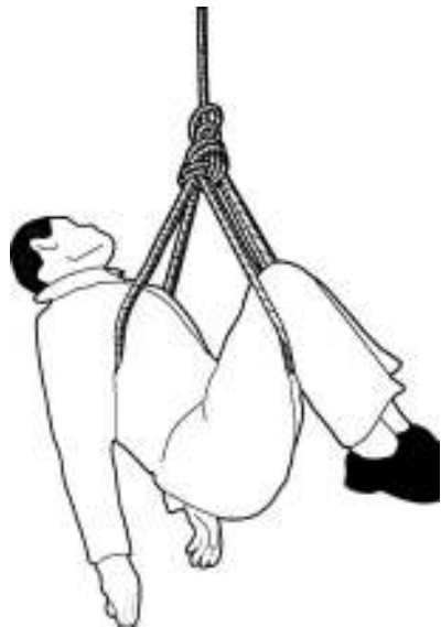
FIGURE 7.13 Full body rope harness being used to lift the victim. (Courtesy AVO, International.)
