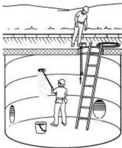
FIGURE 7.9 Vault atmosphere monitoring.
