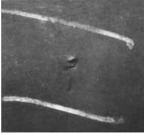
FIGURE 2.40 Protuberance. (Courtesy ASTM.)
