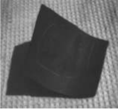
FIGURE 2.42 Repair mark. (Courtesy ASTM.)
