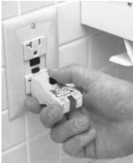
FIGURE 9.13 Receptacle and GFCI tester. (Courtesy Direct Safety Company, Phoenix, Arizona.)
