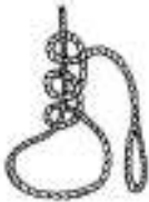
FIGURE 7.10 Securing the victim using a hand line.
