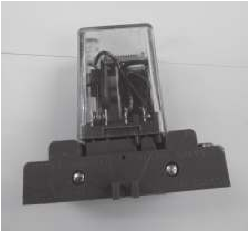
FIGURE 10-3 “Ice-cube” relays and plug-in bases for easy replacement.
