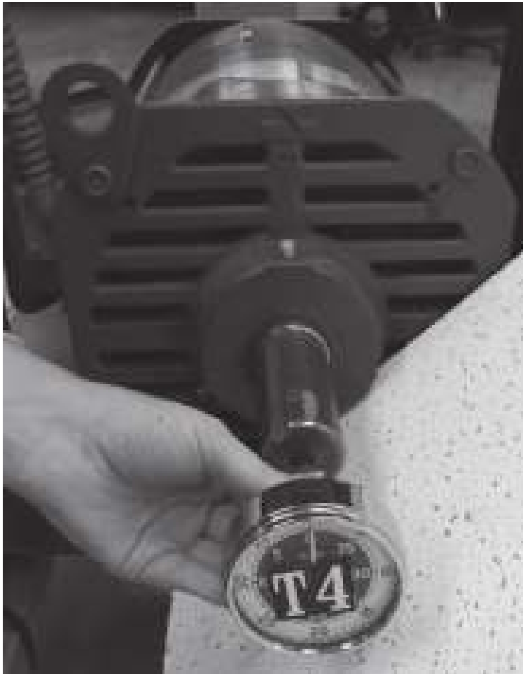
FIGURE 25-6 Mechanical tachometer used to measure shaft RPM.
