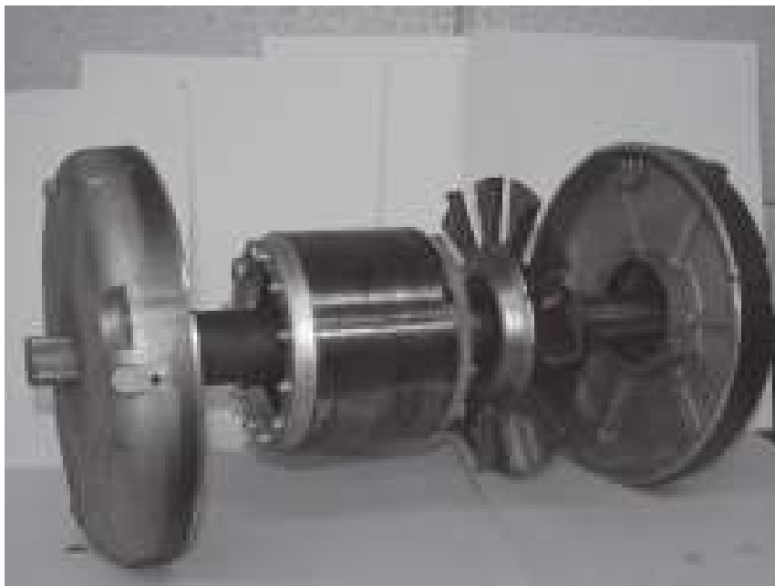
FIGURE 12-3 Squirrel-cage rotor with internal fan and end bells of induction motor.
