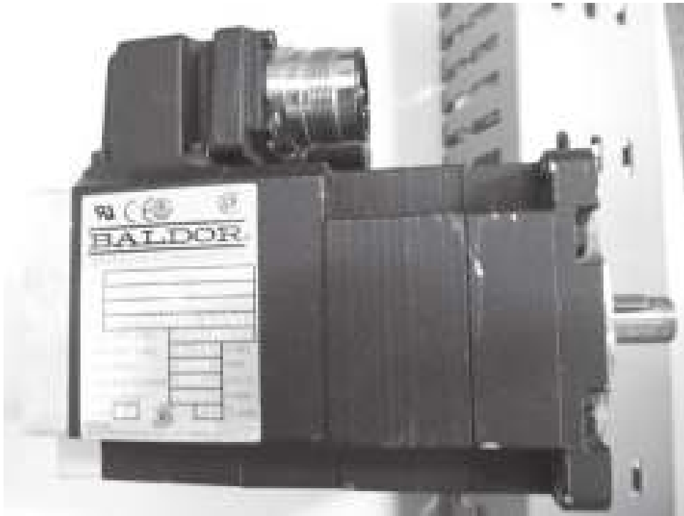
FIGURE 20–3 Servo motor used to produce robot joint movement.
