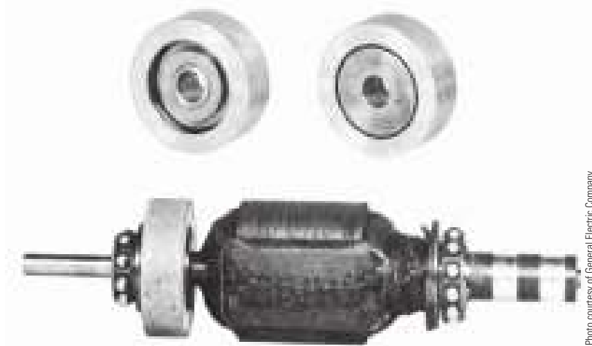
FIGURE 20-12 Wound rotor with oscillation damper and slip rings for selsyn units.
