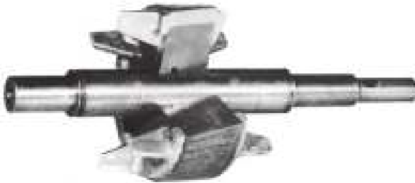
FIGURE 12-6 Cutaway view of a squirrel-cage rotor.
