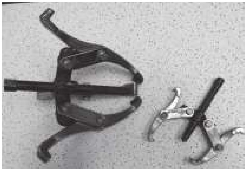
FIGURE 25-8 Bearing pullers. Use jaws to pull bearing off the shaft.
