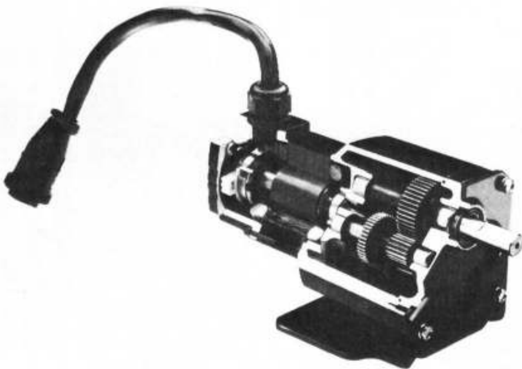
Sectional view of a brushless gearmotor. (Courtesy of Bodine Electric Company)
