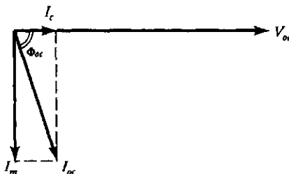
Figure 4.23 The phasor diagram of a two-winding transformer under open-circuit test.
