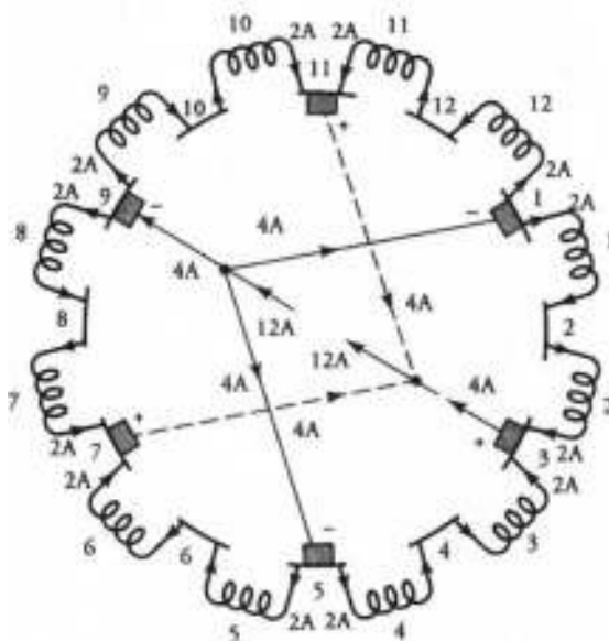
Figure 5.7 Brush connections and currents in six parallel paths of a lap-wound machine of Figure 5.6 when operated as a dc generator.
