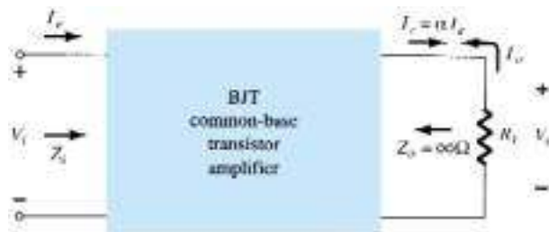
Figure 7.19 Defining A_v = V_o/V_i for the common-base configuration.
