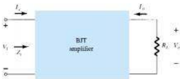
Figure 7.15 Determining the loaded current gain.
