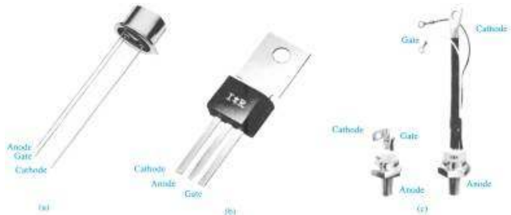
Figure 21.10 SCR case construction and terminal identification. [(a) Courtesy General Electric Company; (b) and (c) courtesy International Rectifier Corporation.]
