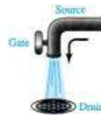
Figure 5.3 Water analogy for the JFET control mechanism.
