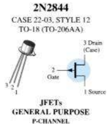
Figure 5.19 Top-hat container and terminal identification for a p-channel JFET.
