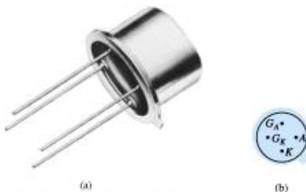
Figure 21.20 Silicon-controlled switch (SCS): (a) device; (b) terminal identification. (Courtesy General Electric Company.)
