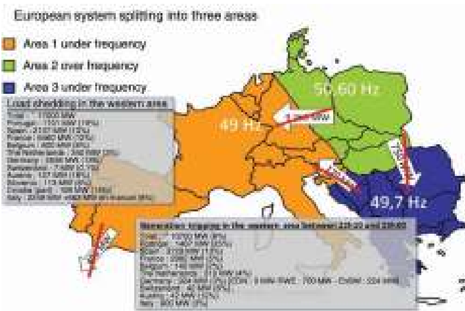
Figure 13.24. Schematic map of UCTE area split into three areas and load shedding in the western area [25,26,29].
