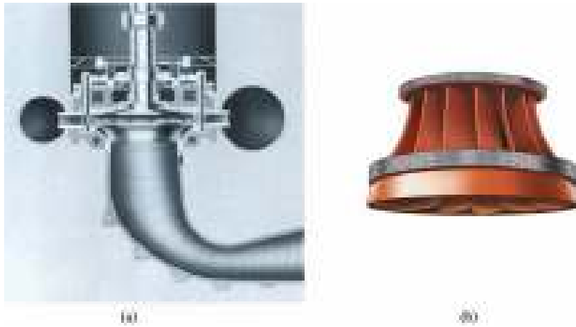
Figure 3.7. A typical vertical shaft reaction turbine arrangement.
