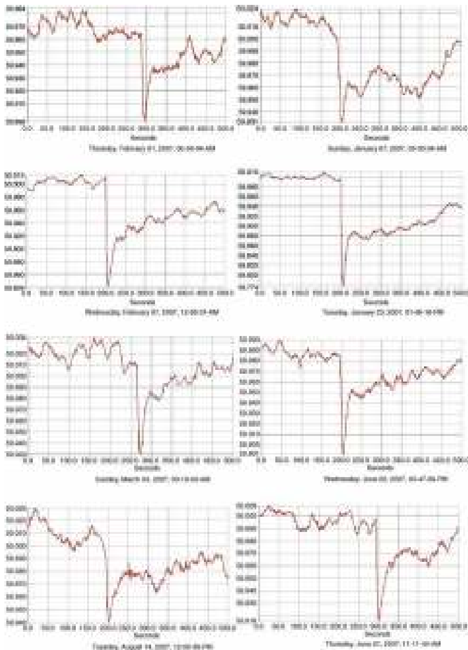
Figure 6.50. Typical frequency time responses in the WECC of large generation trips.
