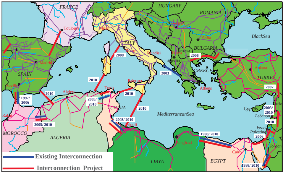
Figure 9.72. The MEDRING Power System.
