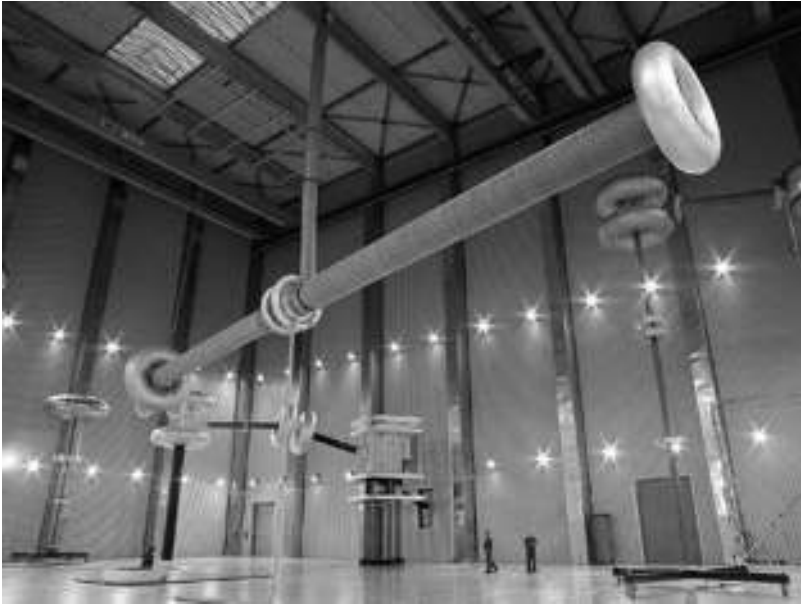
Figure 12.19 Bushing tests at HSP Laboratory, Cologne
