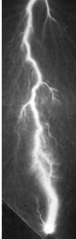
Figure 19.13 Lichtenberg figure of leaders
