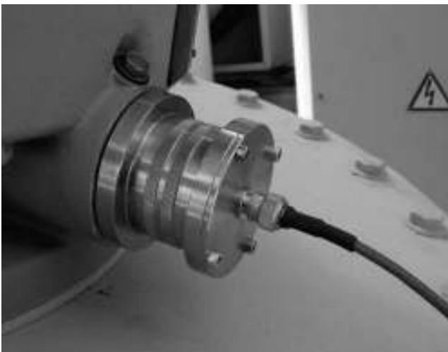
Figure 20.5 Probe connected directly to bushing tap (courtesy of Alstom Grid)
