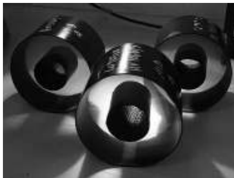
Figure 6.4 Samples of XLPE insulation made temporarily transparent for quality control checks by heating in an oil bath
