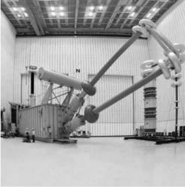
Figure 12.18 800 kV DC resin-impregnated paper bushings
