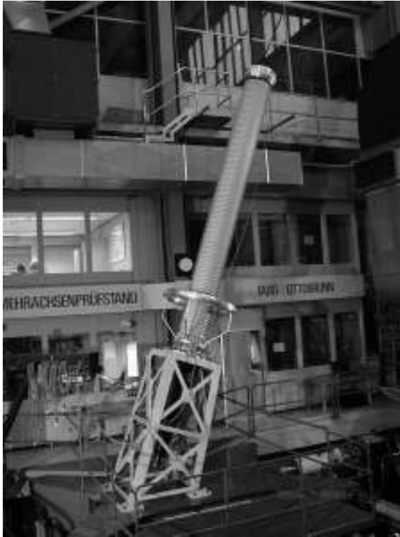
Figure 12.20 Seismic withstand test on polymer transformer bushing
