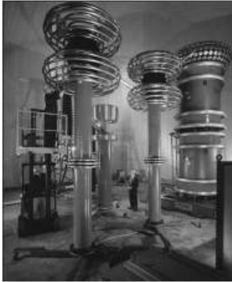
Figure 6.16 Resonant test system for 650 kV, 31 A AC
