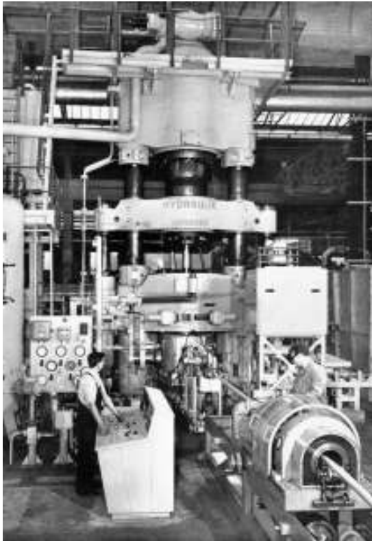
Figure 6.7 An aluminium extruder and corrugator for applying corrugated seamless aluminium sheathing
