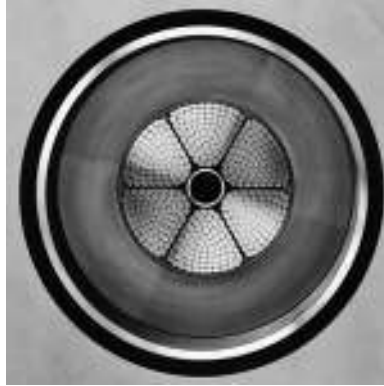
Figure 6.3 Cross section of a Milliken-conductor paper-insulated fluid-filled corrugated aluminium-sheathed cable
