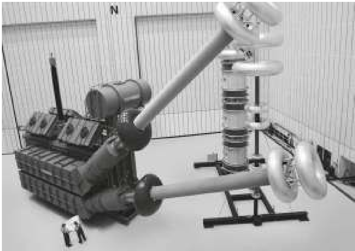
Figure 7.2.3-2: The world's first 800 kV HVDC converter transformer with AC bushing (left, in an upright position) and HVDC bushings for both the winding terminations on the converter side (in the foreground and in an inclined position) after the final acceptance tests in the high voltage test field [453] (5000 MW HVDC system Yunnan-Guangdong in the southwest of China, photo Siemens).
