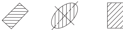
Fig. 2.11 Preferred hatching angles
