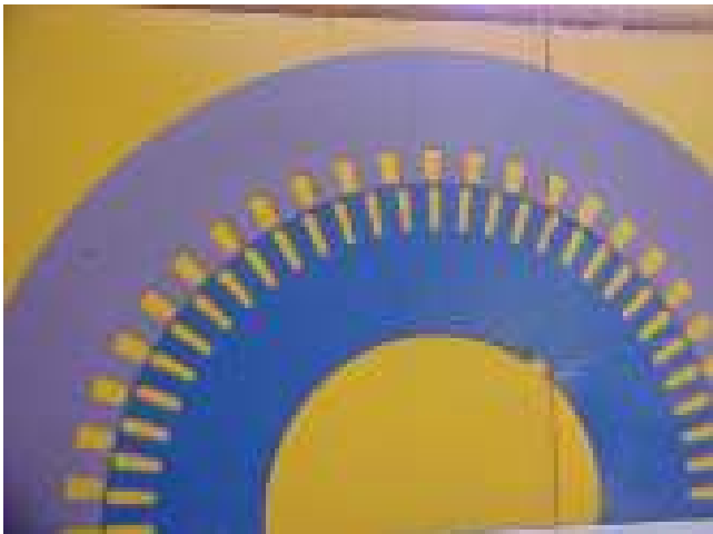
FIGURE 6.15 Stator and rotor punchings for a large induction machine. (Courtesy of Equacional Motores, Brazil.)
