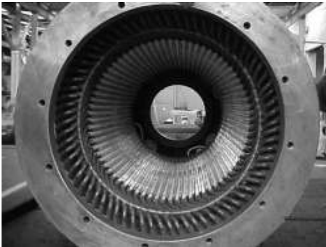
FIGURE 6.13 (See color insert.) Medium-sized eight-pole induction machine, with form wound stator coils. (Courtesy of Equacional Motores, Brazil.)
