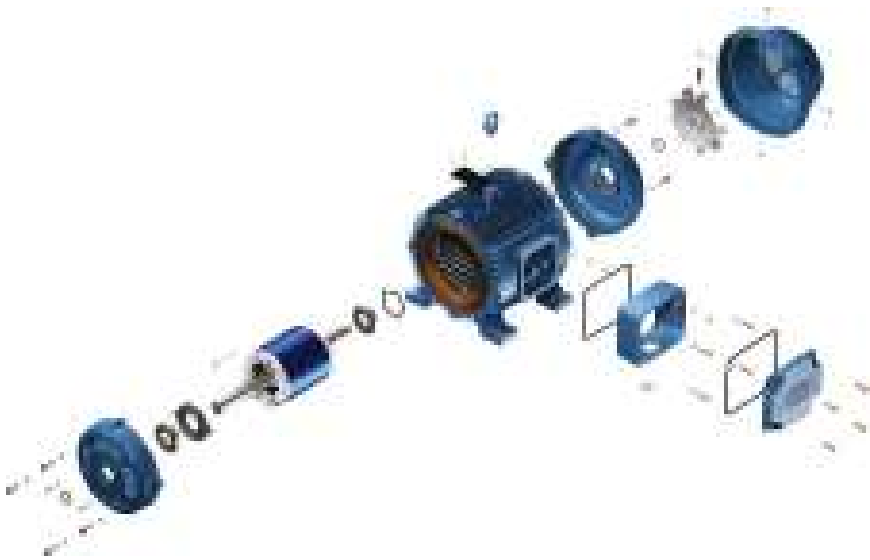
FIGURE 6.2 Exploded view of induction generator major parts. (Courtesy of WEG Motores, Brazil.)
