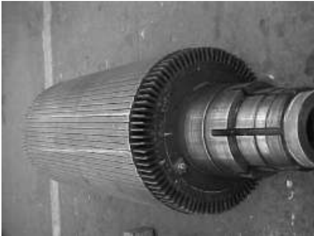
FIGURE 6.17 (See color insert.) Medium-sized squirrel cage rotor winding. (Courtesy of Equacional Motores, Brazil.)
