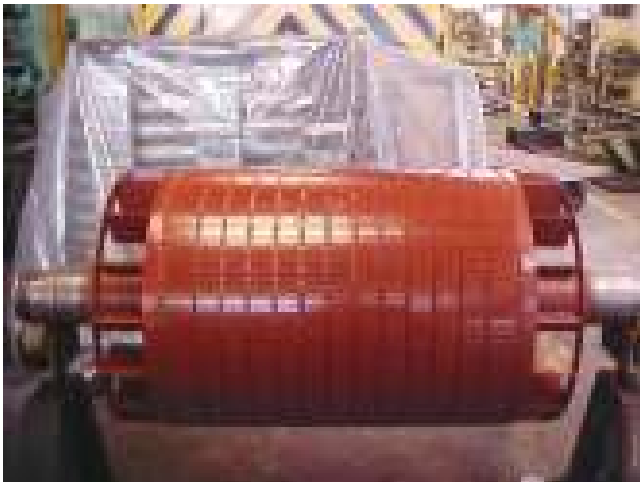
FIGURE 6.4 Finished squirrel cage for large power induction motor. (Courtesy of Equacional Motores, Brazil.)
