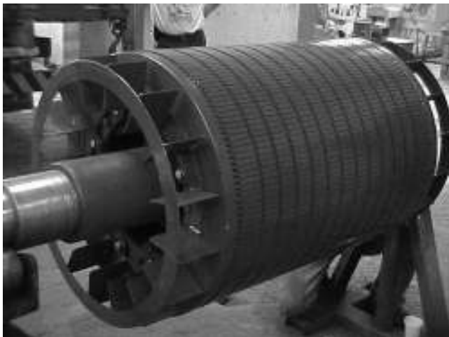
FIGURE 6.14 (See color insert.) Squirrel cage rotor for a large induction machine showing the brazen bars to the end rings. (Courtesy of Equacional Motores, Brazil.)
