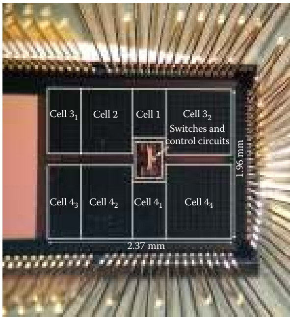
FIGURE 6.13 Recursive switched-capacitor voltage regulator implementation, comprising eight cells of binary weights and two control loops. (a) Block diagram of the overall RSC chip with binary search controller. (b) 4 bit Recursive SC test chip photo.
