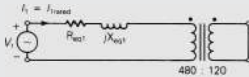
(a) Short-circuit test (neglecting shunt admittance)
