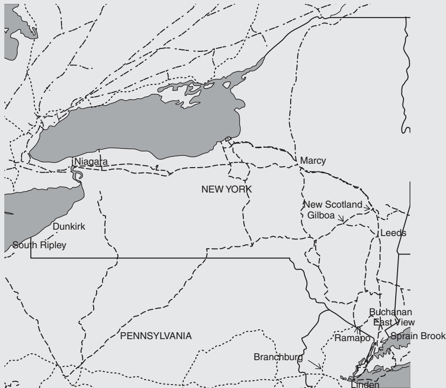
Figure 1 A representation of the New York Power System (green lines indicate 765 kV, orange lines indicate 500 kV, and red lines indicate 345 kV)
