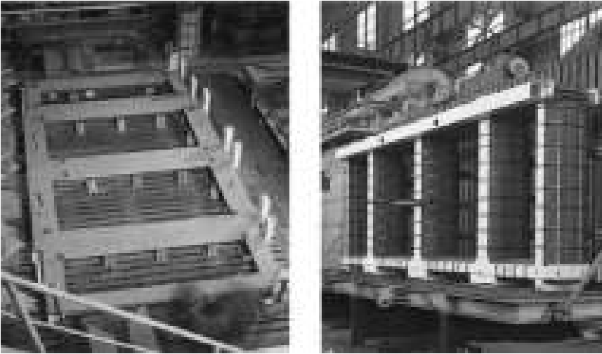
FIGURE 4.18 Five-legged transformer (Alstom 600 MVA transformer).
