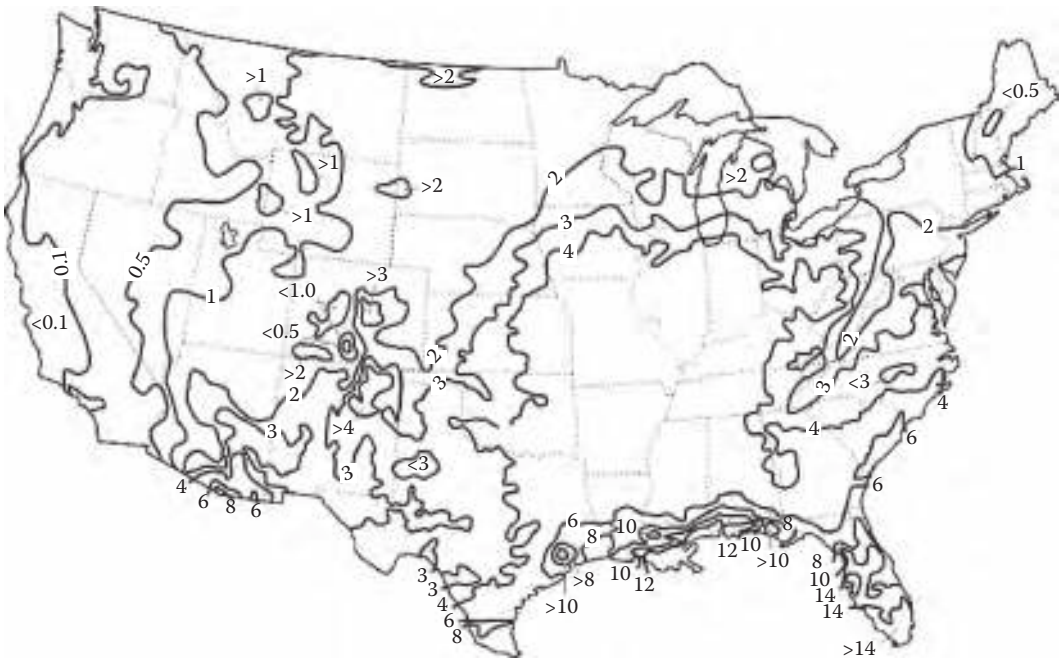
FIGURE 6.3 Ten-year average GFD map of the United States. (Reproduced from Vaisala, Inc. of Tucson, AZ., Standards Information Network, How to protect your house and its contents from lightning, IEEE Guide for Surge Protection of Equipment Connected to AC Power and Communication Circuits , IEEE Press, New York, 2005. With permission.)
