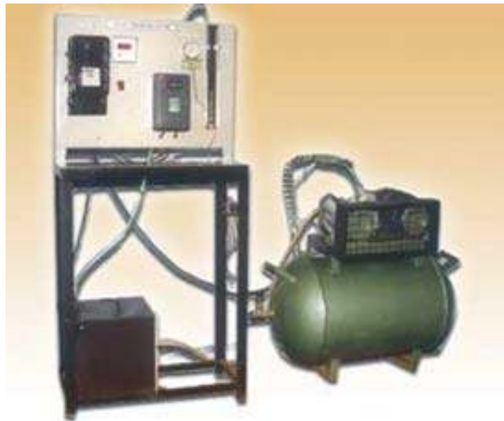
Measuring efficiency of compressor.
