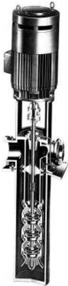
Figure 4.35 Vertical turbine pump mounted in a barrel can be used for high-pressure suction sources, or for pumping from vessels below atmospheric pressure. (Courtesy of Goulds Pumps, Inc., ITT Industries, Seneca Falls, NY.)
