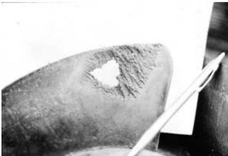
Figure 2.10 Material loss from impeller vane due to cavitation.
