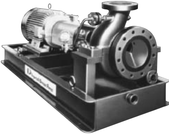
FIGURE 98 Horizontal shaft overhung pump and driver on a structural steel bedplate with a raised edge around the base and a tapped drainage connection (Flowserve Corporation)
