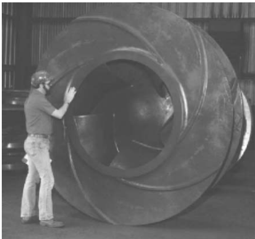
FIGURE 2 Dredge pump impeller, 105 in (2.67 m) diameter
