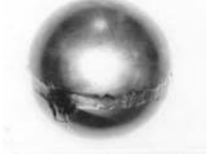
FIGURE 14 Erosion damage of an AISI-type, 440C stainless steel ball valve in a coal slurry service
