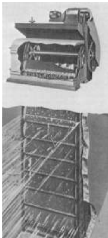
FIGURE 11 Traveling water screen (Envirex Inc., a Rexnord Company)
