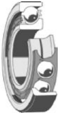
FIGURE 89 Single-row, angular contact bearing (SKF USA, Inc.)
