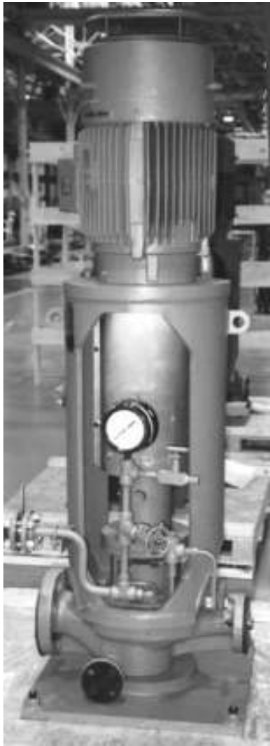
FIGURE 6 Single stage, overhung, vertical inline pump with separate bearing frame—API 610 Type OH3 (Flowserve Corporation)
