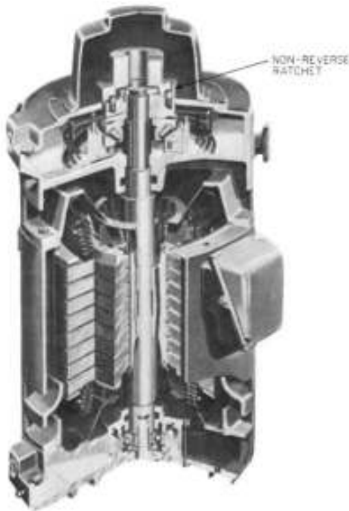
FIGURE 18 Section of vertical hollow shaft motor showing nonreverse ratchet. Spring-loaded pins ride on ratchet plate in one direction only (General Electric).
