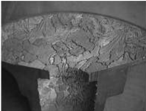
FIGURE 6 The surface of a stuffing box cover that experienced intergranular corrosion due to sensitization. The grains are clearly evident on the interior of the bore as well.
