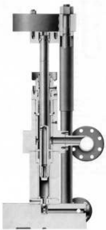
FIGURE 5 Special high-pressure liquid-end designs arrange the suction and discharge valves on the same axis as the plunger, thus eliminating intersecting bores (Flowserve Corporation).
