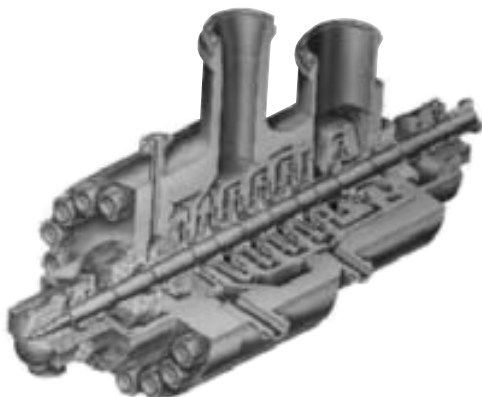
FIGURE 22 Double-casing multistage pump with radially split inner casing (Flowserve Corporation)
