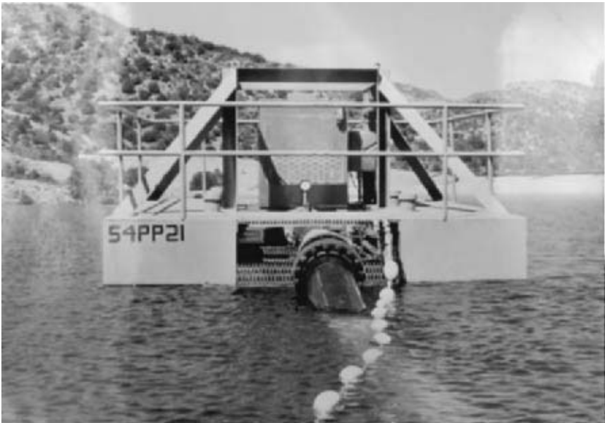
FIGURE 7 Unique design float-mounted pump (Hazleton Pumps, Inc.)
