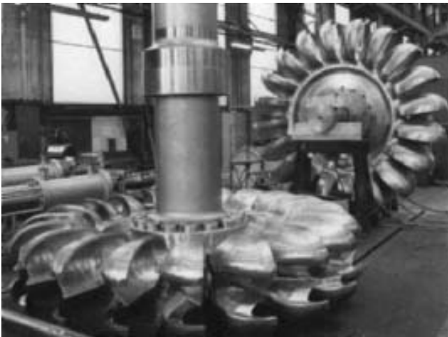
FIGURE 7 Impulse (or Pelton) runners (Voith Siemens Hydro)
