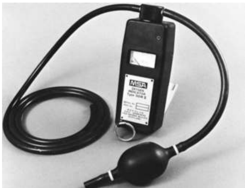
Figure 3.3.11 Portable oxygen analyser (Courtesy M.S.A. Ltd)
