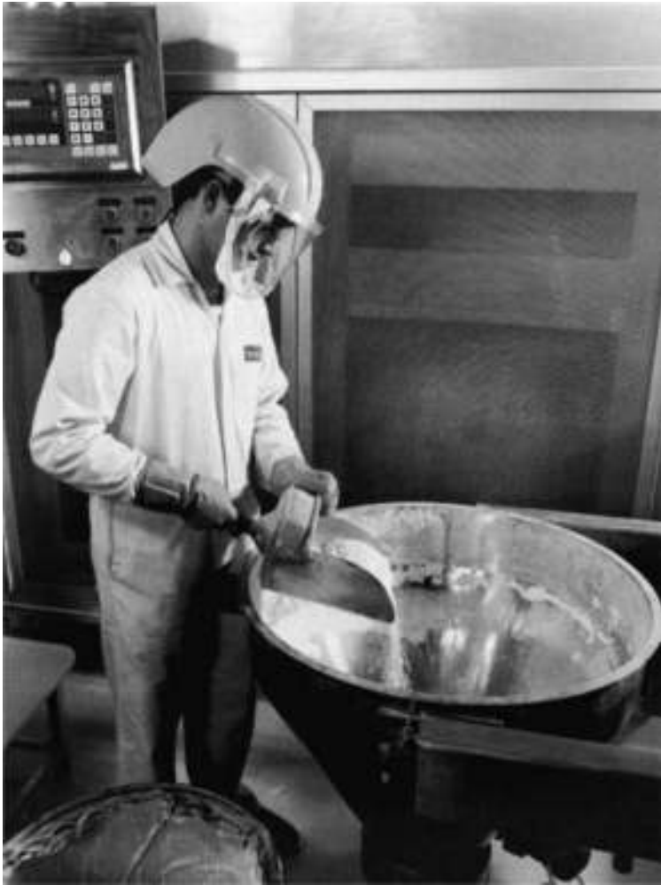
Figure 4.7.2 Protective clothing to provide protection against contact and dust (Courtesy Rhone-Poulenc-Rorer)
