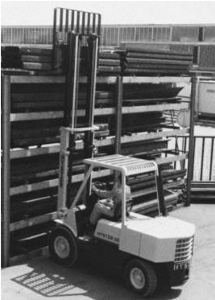
Figure 4.3.15 High lift fork truck with load rest, overhead and rear guards (Courtesy Hyster Europe Ltd)
