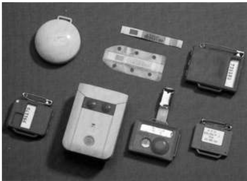
Figure 3.4.2 Devices for monitoring the exposure of workers to various types of radiation. (Courtesy NRPB)
