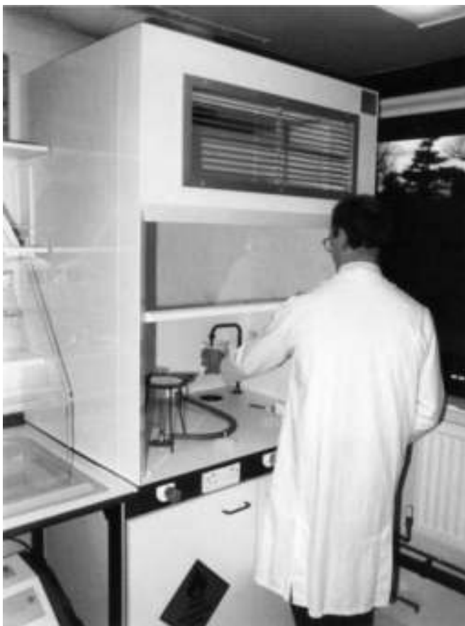
Figure 4.7.7 Well ordered fume cupboard (Courtesy British Sugar plc)
