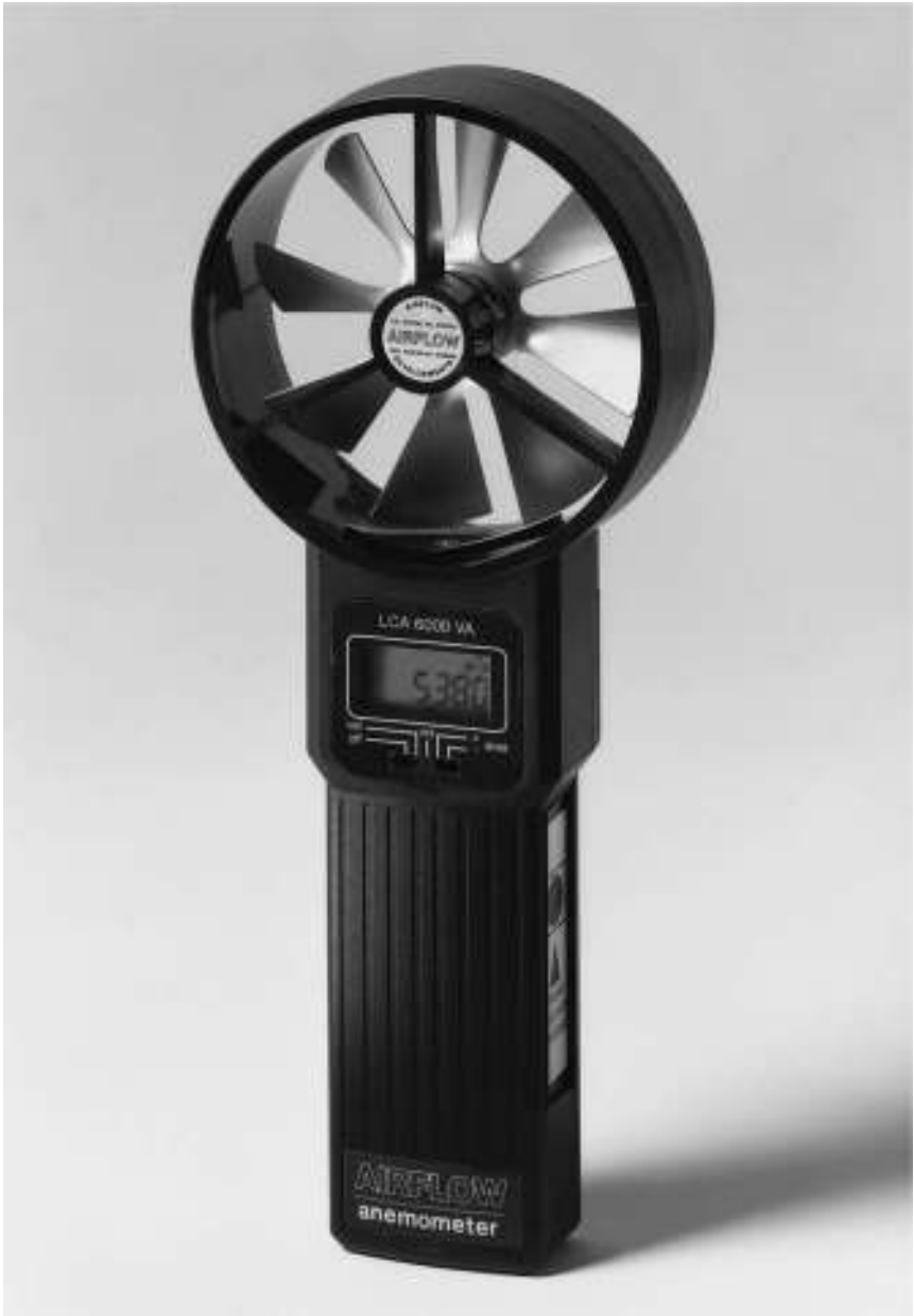
Figure 3.6.7 Vane anemometer (Courtesy Air Flow Developments Ltd)
