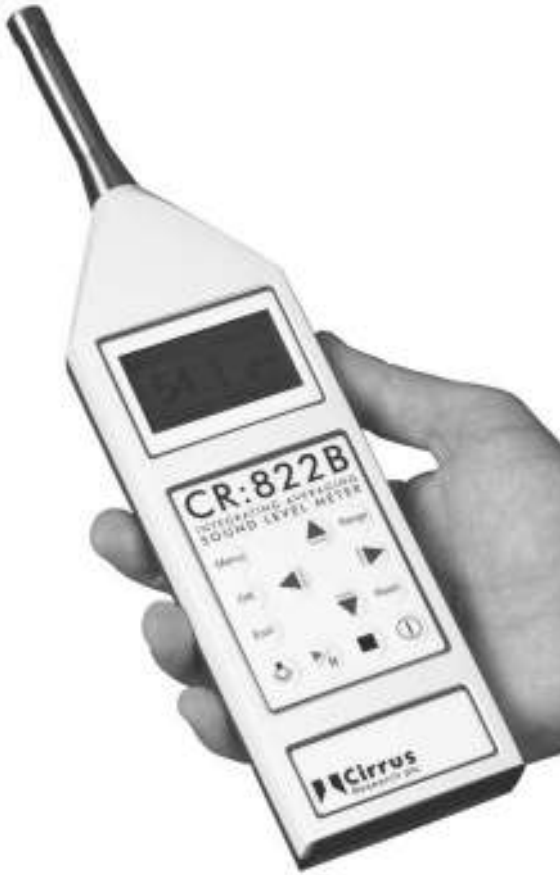
Figure 3.5.6 Industrial hand-held sound level meter (Courtesy Cirrus Research plc)
