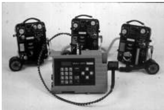
Figure 3.3.9 Organic vapour analyser (Courtesy Quantitech Ltd)
