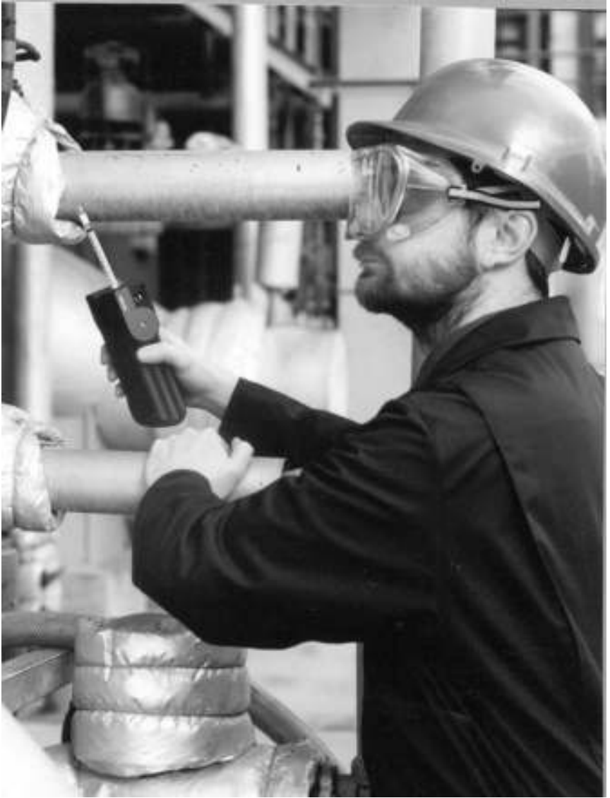
Figure 3.3.2 Stain detector tube and hand pump (Courtesy Draeger Safety Ltd)
