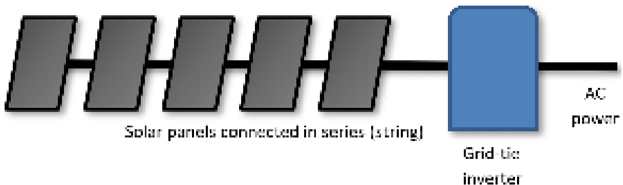
A simplified block diagram showing the basic layout of a high voltage in-series solar energy system
