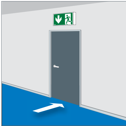
At each exit door
