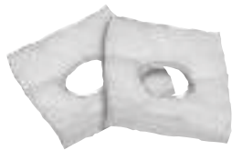
Step 1 Layer batting and variable conductor sizes to be welded into dry mould
