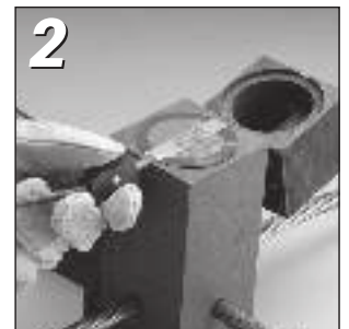
2 Attach control unit termination clip to ignitor strip
