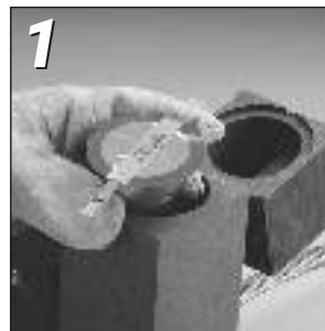
1 Insert Cadweld Plus package into mould
