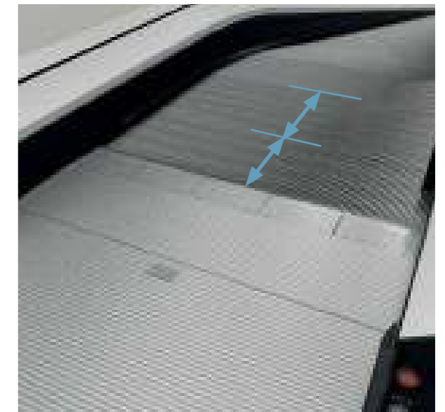
Figure 5.12 The number of horizontal pallets required for inclined autowalks varies with the speed and inclination (one horizontal pallet on the top, two horizontal pallets on the bottom picture).
