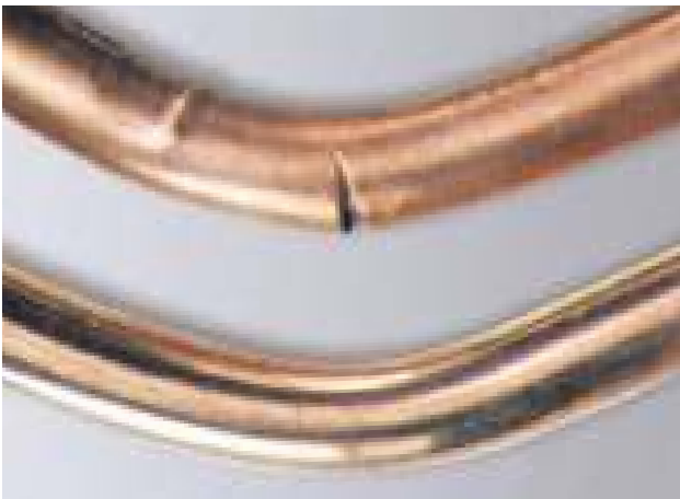
Figure 76. Copper bonded and copper clad earth rods.
