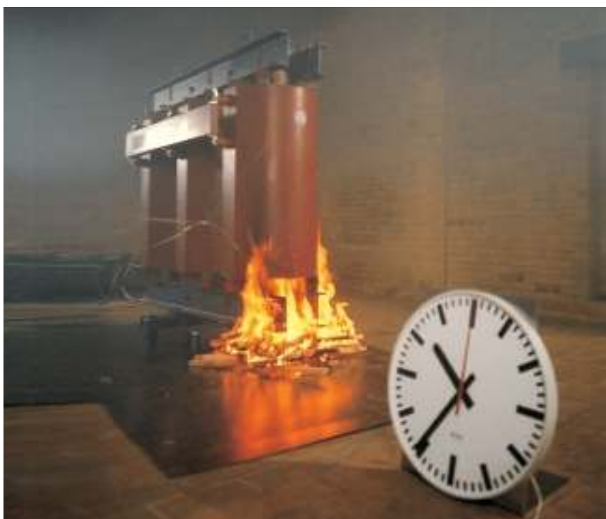
Fig. 51: Flammability test of cast-resin transformer
